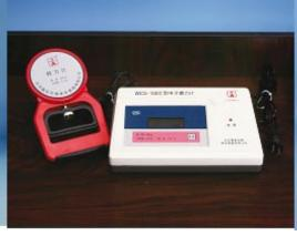
Picture 2-11 Grip dynamometer
