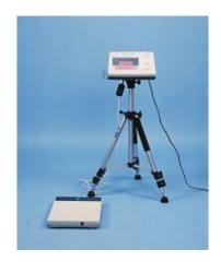
Picture 2-2 Electronic digital scale
