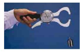
Figure-4 Checking the skinfold thickness caliper
