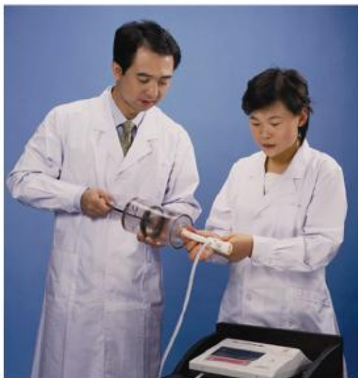
Figure 1-2 Calibration of electronic spirometer
