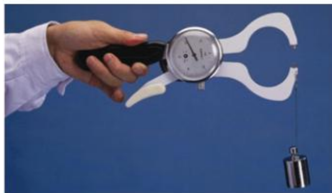
Figure 1-3 Calibration of skinfold caliper
